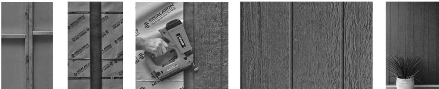
Fixings must be provided at 200mm centres to the studs and plates nearest the edge of the sheet, and 200mm centres throughout the centre of the sheet to all underlying studs and noggings. Fixing shall be no closer than 12mm from the sheet edges and must not be in the grooves of the sheets. Drive fixings flush with the sheet surface. No punching is permitted. Refer to the fixing details for pre-primed Weathergroove.
