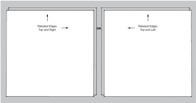
Establish a horizontal datum line where, as a minimum, the bottom edge of the sheet overhangs the bottom plate by 20mm. Plan sheet layout with the rebated faces either:
