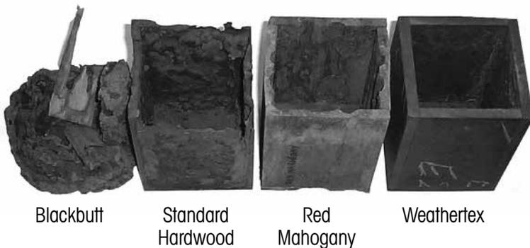
**Samples removed from Termite Test
